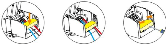
Push the wire pressing board to fix the wires.
