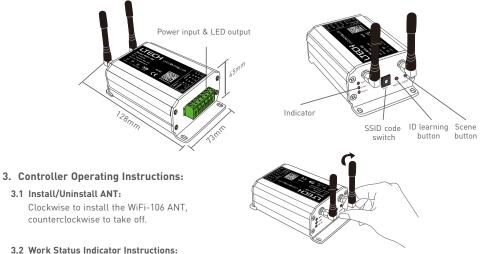
RUN: The indicator light flashes quickly about 60 seconds during the electric initialization. Return to flash slowly after initialization.
