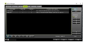
6.7 Click the tab of "DMX devices", set port status to "ON" if connected successfully. Now, you can use computer to control lamps via ArtNet-SPI-1.
