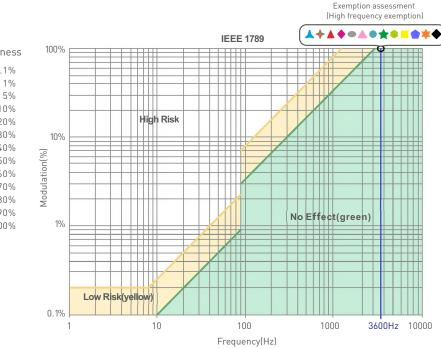
Marks in the right chart are tested results of different current level. The output frequency is 0Hz in 100% brightness and its corresponding modulation is 0%, which could not be shown in the right chart.
