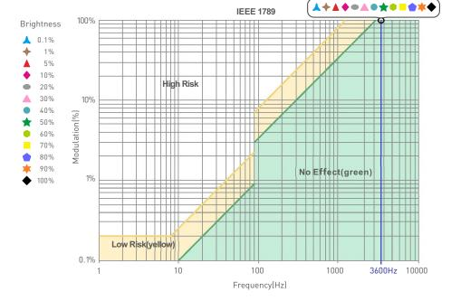
Marks in the right chart are tested results of different current levels. The output frequency is 0Hz in 100% brightness and its corresponding modulation is 0%, which could not be shown in the right chart.
