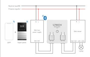
Note: The wireless module and the DALI master cannot be connected together to the same bus.
