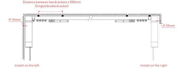
2. If you install a single curtain track, the total width should be no less than 120mm; If you install double curtain tracks, the total width should be no less than 220mm. The width can be adjusted according to the thickness and material of your curtain fabrics and your design.
